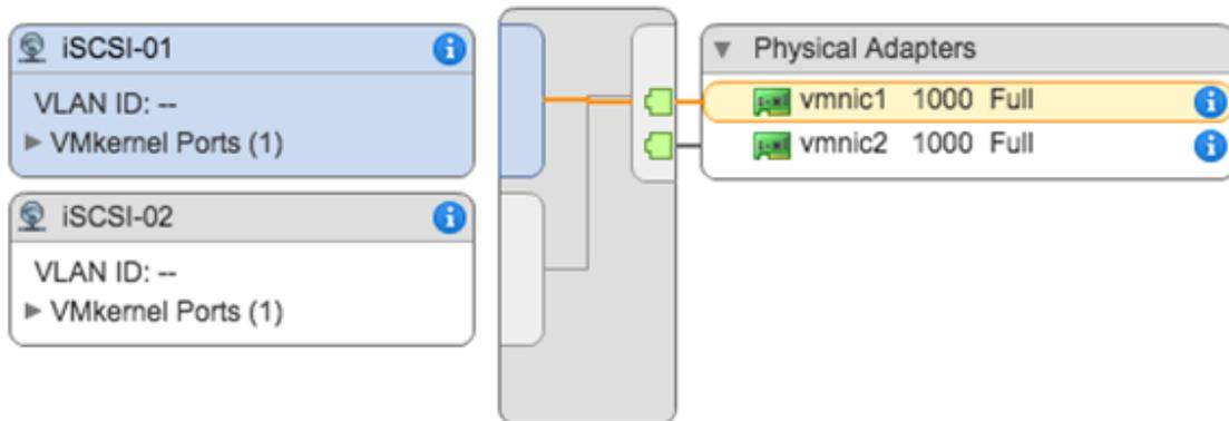
Figure 7 - Single VSS with Two VMkernel Ports
