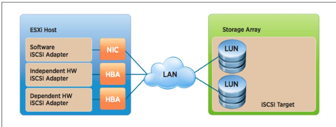
Figure 4 - Software and hardware iSCSI initiators
